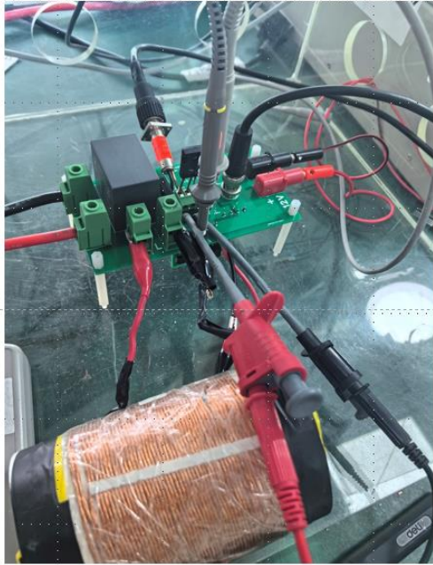
Figure 3: Double pulse testing parameters and PCB for the 1200V TO247-4.
